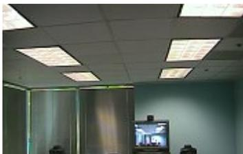
Another one of the biggest issues of lighting is the fluorescent overhead lighting in most office environments. The "ice cube tray" lighting was designed to provide a good source of overhead lighting to illuminate documents and materials on your desk. However, the overhead lighting can cause undesirable shadows to appear on your face - creating especially dark circles under your eyes.
