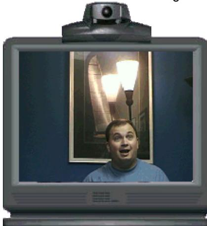
If you include the ceiling and lights in the field of view, the camera will iris down to accommodate the bright lights.
